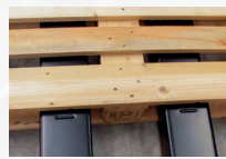
Marking on forks for optimum positioning of the lift truck when laterally lifting a pallet
